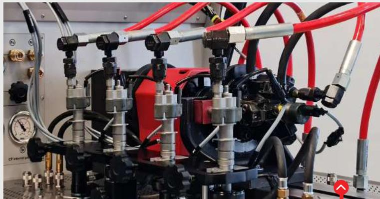
**1 Diesel CRDI testing and coding:**
